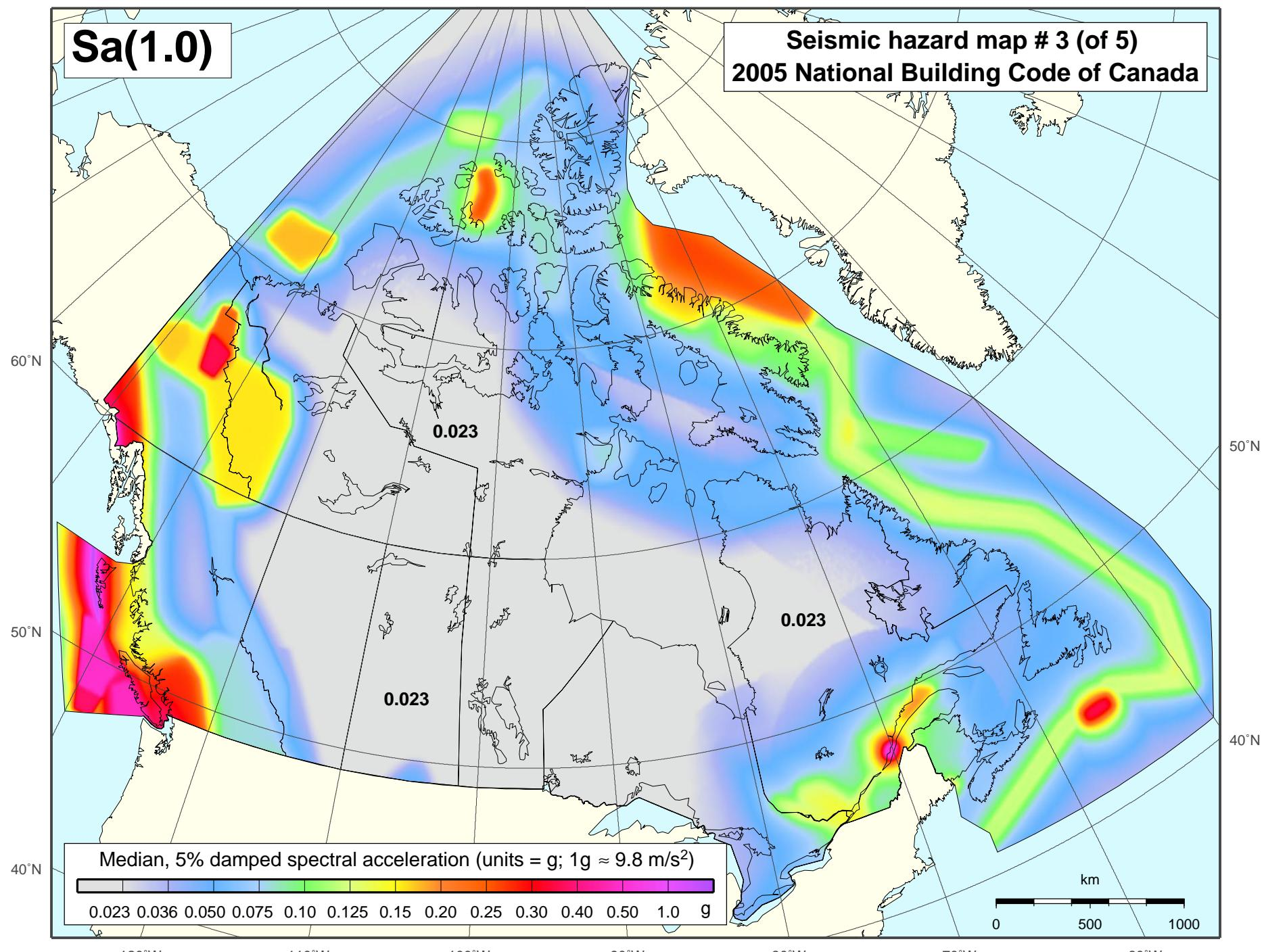
Spectral acceleration for a period of 1.0 seconds at a probability of 2%/50 years for firm ground conditions (NBCC soil class C).
