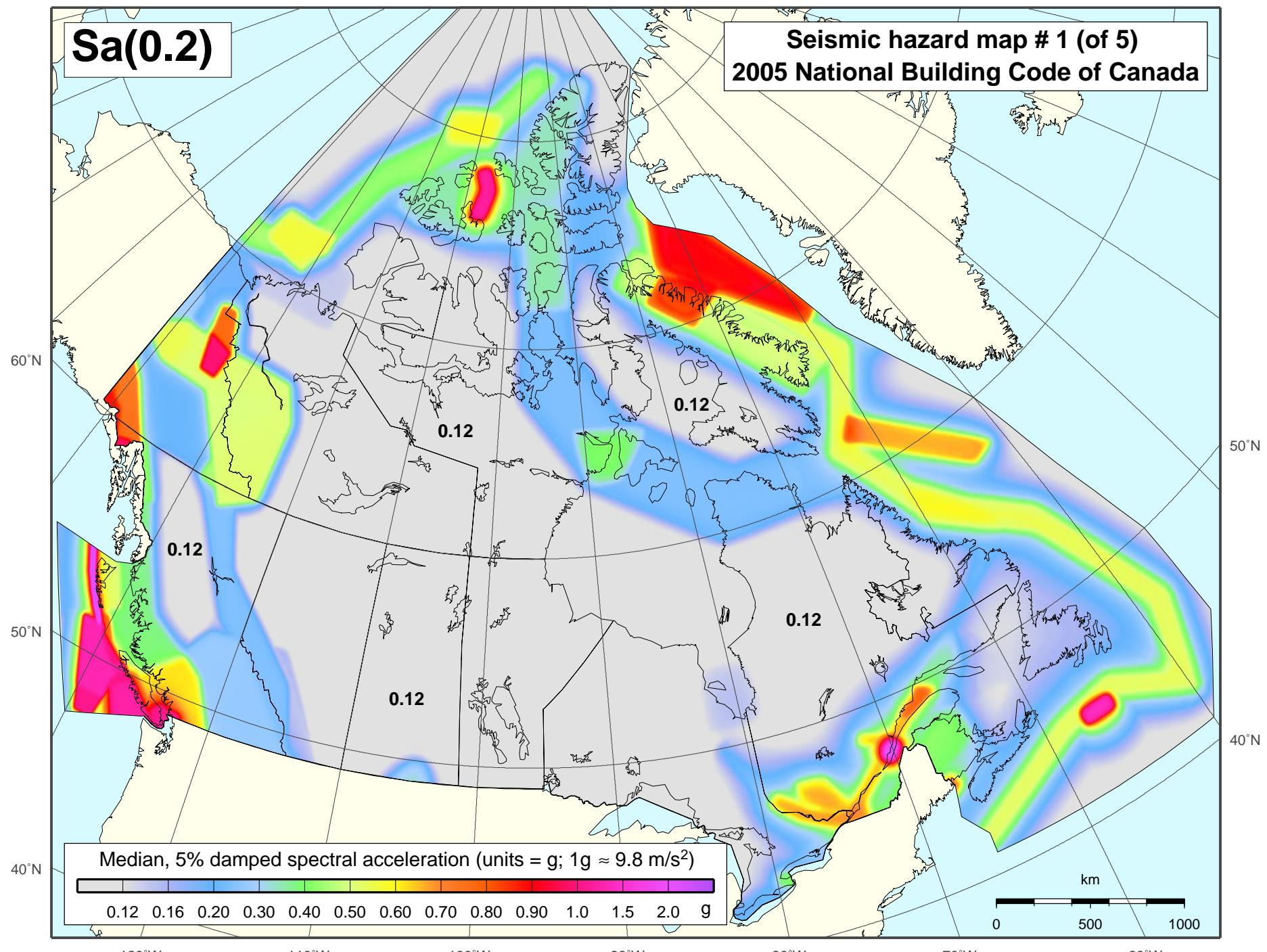
Spectral acceleration for a period of 0.2 seconds at a probability of 2%/50 years for firm ground conditions (NBCC soil class C).
